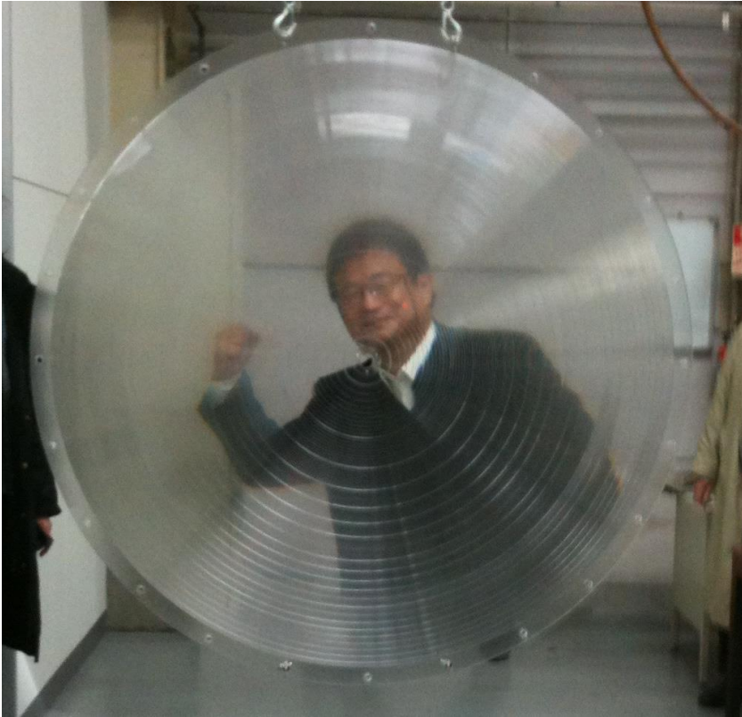
Experimental Fresnel lens with diameter of 1.5m
