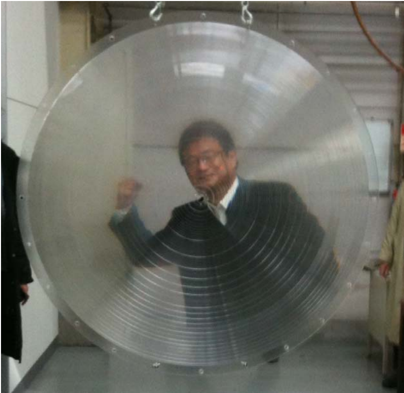
Experimental Fresnel lens with diameter of 1.5m
